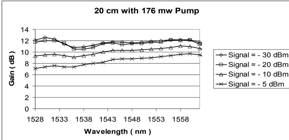
Fig. 3: Flat gain spectrum for 20 cm long waveguide
