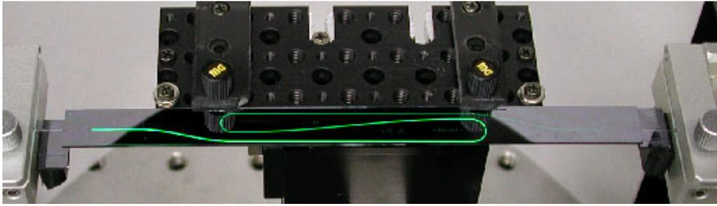
Fig. 1: 4-channel S-shape waveguide array on a 12 cm die
