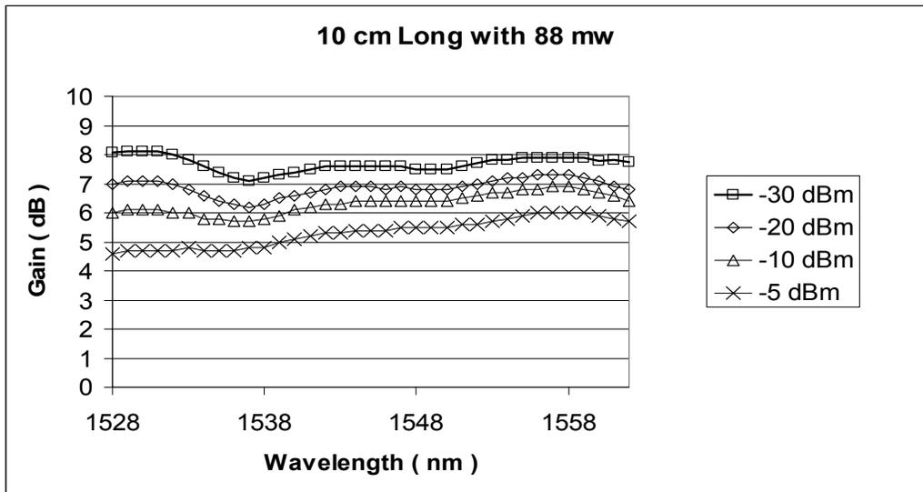
Fig 4: Gain spectrum for 10 cm long waveguide
