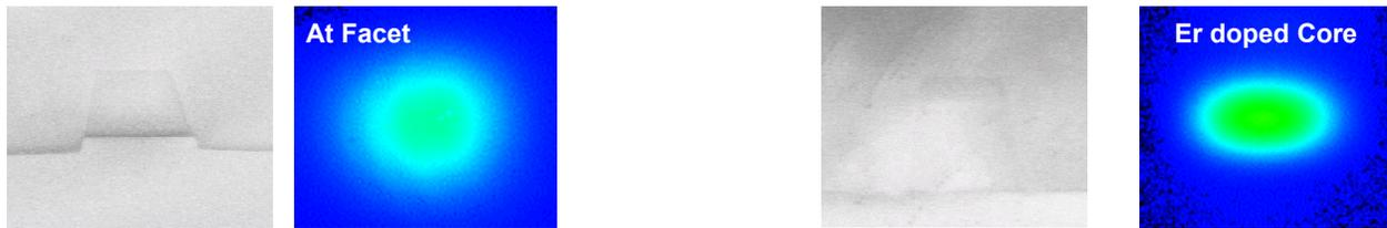
Fig. 2: 980nm pump mode images and SEM cross sections at facet and in the middle of Er-doped waveguide
